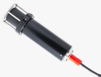
The S2C T "tiny" modems are the new generation light and ultra-compact form factor that represents a size reduction of almost 20% compared to our M-series mini-modems.
